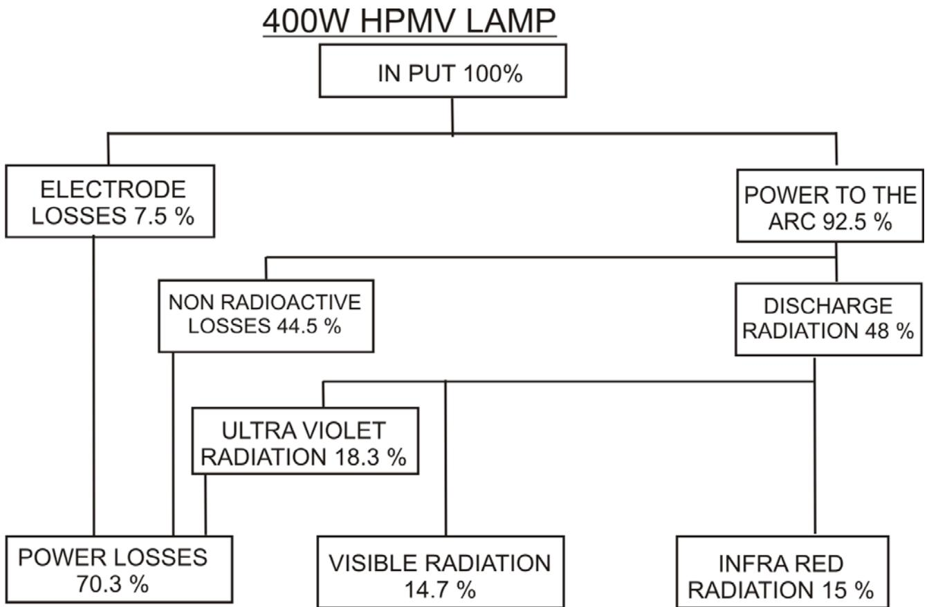
Fig. 3 Energy Balance of HPMV Lamp
