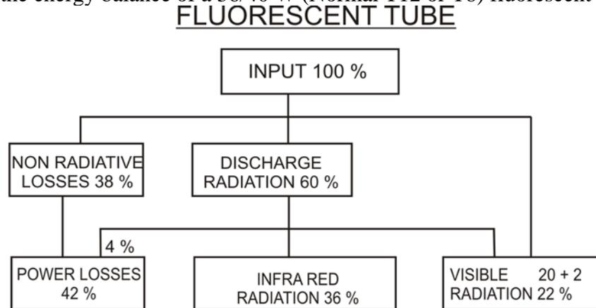
Fig. 2 Energy Balance of Fluorescent Tube
