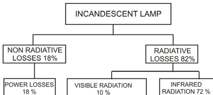
Fig. 1 Energy Balance of Incandescent Lamp
